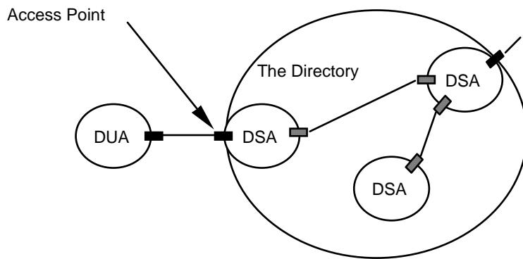
Figure 1: Subsystems in the OSI directory system [X.500 88]
